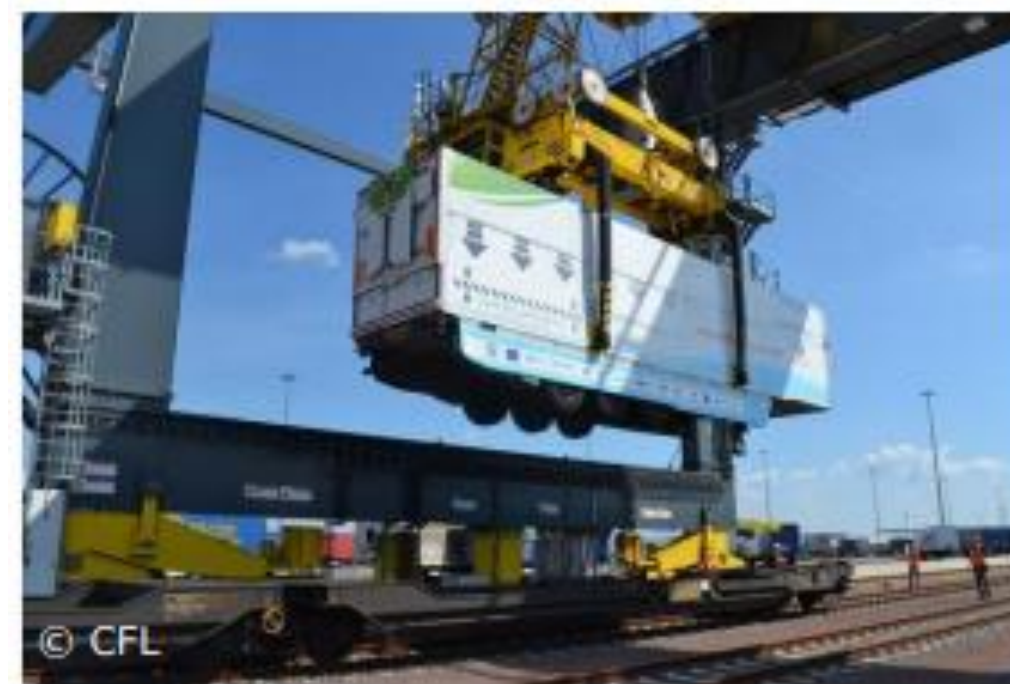
Example of a vertical transshipment operation at Bettembourg terminal
